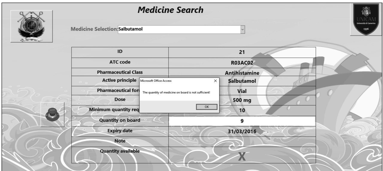
Figure 4. A screenshot of the non-blocking warning created automatically by the software to alert the user that the quantity on board is less than minimum required by regulations
